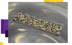
Syntactic foams — strong, exceptionally light materials made of plastic perfused with hollow microspheres — are used in everything from buoys and boat hulls to soccer balls and solid rocket boosters. They are now making their way into new industries, including the automotive sector, but producing the foams at such a large scale is a daunting challenge.
