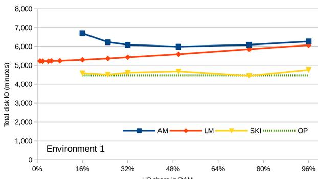
Fig. 3. Total running time in minutes with various UB sizes for medium query rate on SSD. Lower is better.
