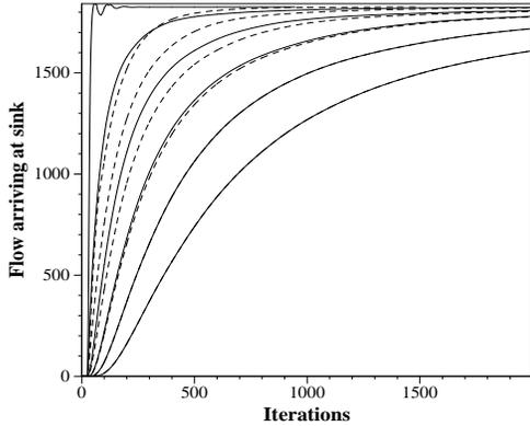
**Fig. 4.** Convergence of the idealized (solid lines) and realistic (dashed lines) second-order method with  $\beta$  equal to 1.0 (lower curve), 1.2, 1.4, 1.6, 1.8, and 1.95 (upper curve). Note that the two lowest dashed curves are hidden by the corresponding solid curves.
