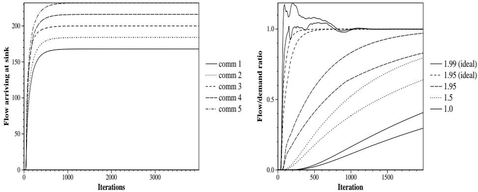
**Fig. 6.** Convergence of the idealized second-order method with  $\beta = 1.95$  on an RMF graph with five commodities.
