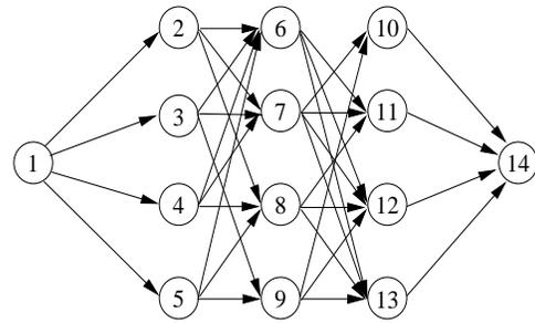
**Fig. 12.** Random leveled graph with 3 levels and 14 nodes. All edges have randomly chosen capacity, except for edges connecting to the source or sink, which have capacity large enough such that they never constitute a bottleneck.
