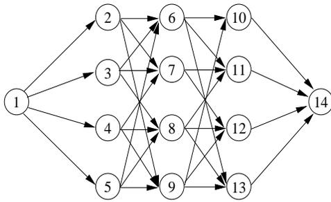
**Fig. 11.** Mesh graph with 3 levels and 14 nodes. All edges have randomly chosen capacity, except for edges connecting to the source or sink, which have capacity large enough such that they never constitute a bottleneck.
