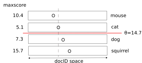
Figure 1: Pivot selection in the WAND algorithm with 4 terms, where the current threshold for the top- k results is 14.7. The list for cat is selected as pivot since 10.4 + 5.1 > 14.7 .
