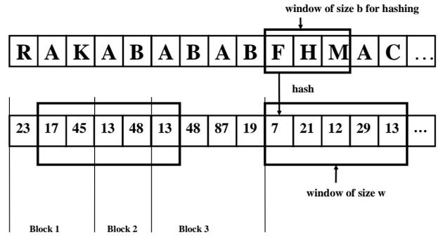
**Figure 2.1: Example of the winnowing approach on a file. A small window of size  $b = 3$  moves over the file to create a sequence of hashes. A larger window of size  $w = 5$  moves over the hashes to determine block boundaries.**
