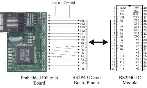
Figure 4: Pin connections between the EEB to BS2P40
