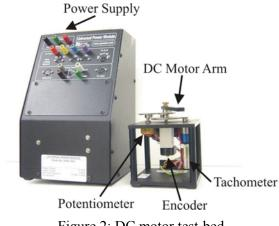
Figure 2: DC motor test-bed
