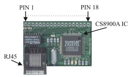
Figure 3: The embedded ethernet board
