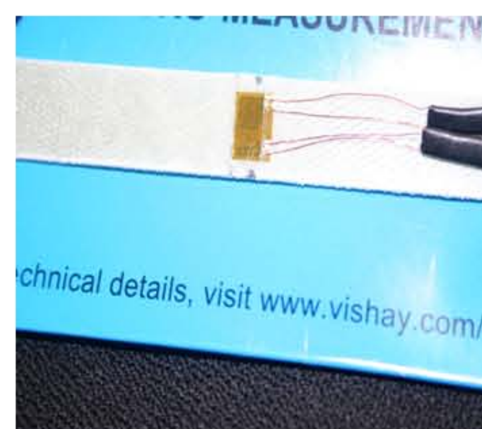
Fig. 8. Strain gauge bonded to composite specimen using Epoxy
