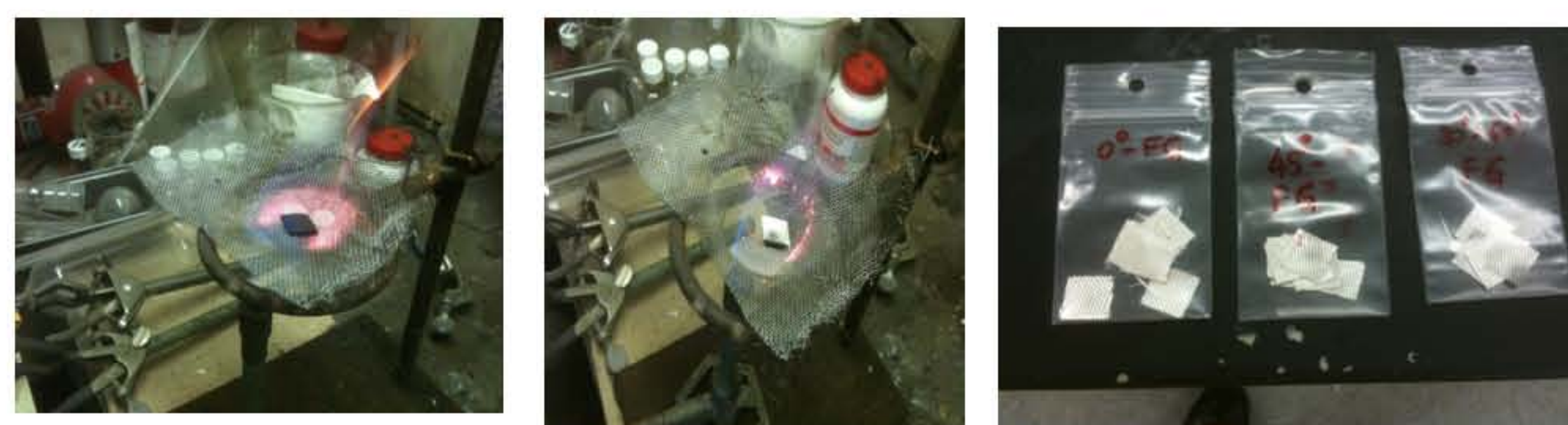
Fig. 7. Burning and recovery of original fiberglass from composite
