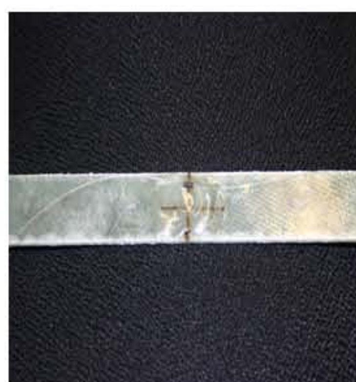
Fig. 11. Composite bonded with optical fiber loop
