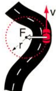
Fig. 3. Centripetal force on a banked curve
