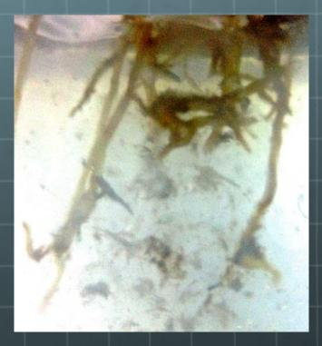
On top of the transparent soil, a thin, metal netting, and dampened cloth were placed to prevent any soil particles from seeping into the beads and clouding our visibility of the roots. A hole, or passageway was created (2.5 cm diameter) to allow growing roots to eventually invade the transparent Aquabeads solution.
