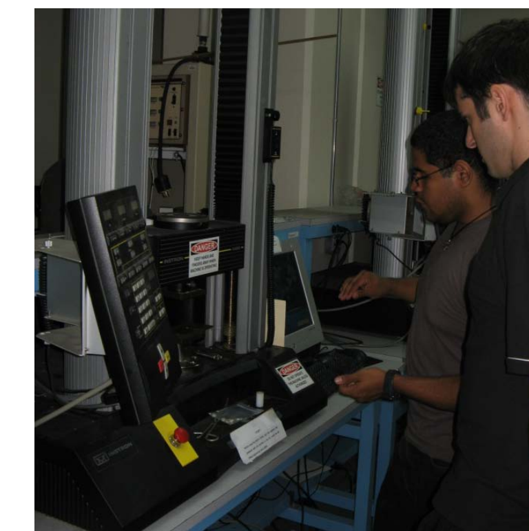
Instron 4469 quasi-static system
