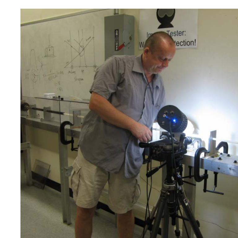
SHPB dynamic system with high speed camera in place
