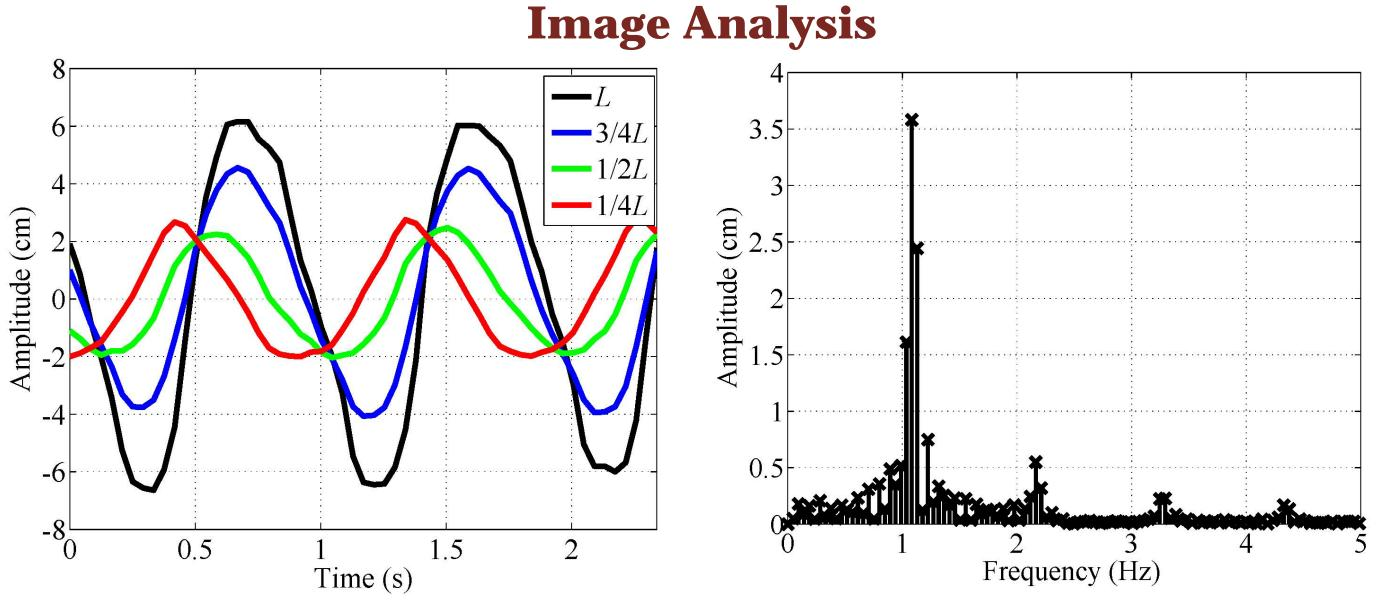
Image analysis was performed using *Xcitex ProAnalyst* to determine the displacement and frequency of oscillation of the realized biomechanical fish tail. Points along the  $\frac{1}{4}$ ,  $\frac{1}{2}$ ,  $\frac{3}{4}$ , and full length of the tail were tracked for a total of 12 periods.
