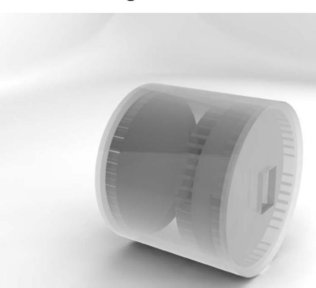
biomechanical tail is The actuated using a water resistant *CS-80* Hobbico Command servomotor. Shown (left) is the computer rendered design of the motor encasement.
