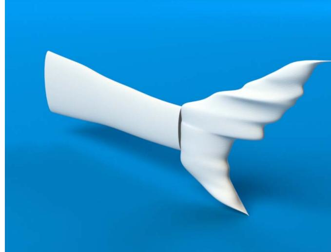
The computer rendered tail section is converted to a computer aided manufacturing (CAM) geometry, shown (right). A slender stainless steel beam is inserted into the mold for structural support.
