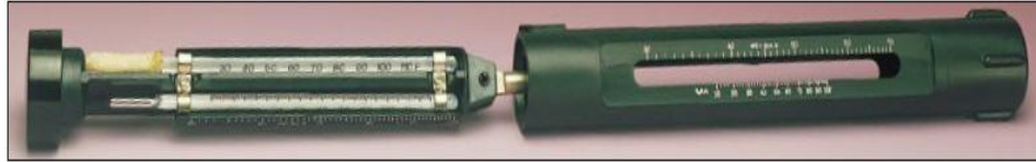
Figure 2. Sling psychrometer for relative humidity measurement. 12, 13
