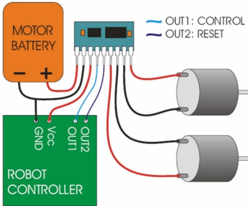
Figure 1 – motor controller diagram
