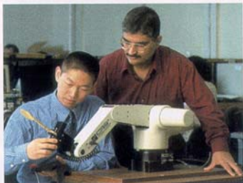
Dr. Vikram Kapila oversees graduate student Hong Wong '01 working on a five degree of freedom robotic manipulator. With funding from NASA, Kapila aims to manipulate spacecrafts in orbit.
