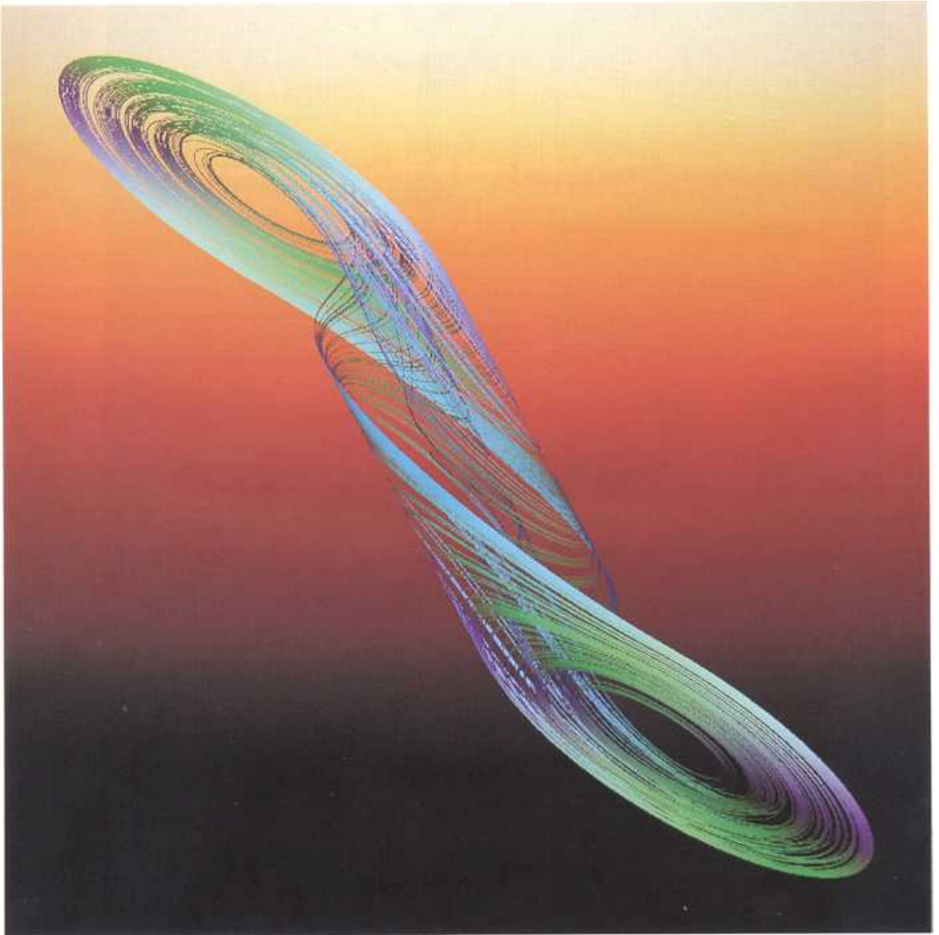
Fig. 4. (b) Computer-calculated chaotic attractor from the dimensionless Chua's Equation (1) with \alpha = 15.6 , \beta = 25.58 , m_0 = -8/7 , m_1 = -5/7 .
