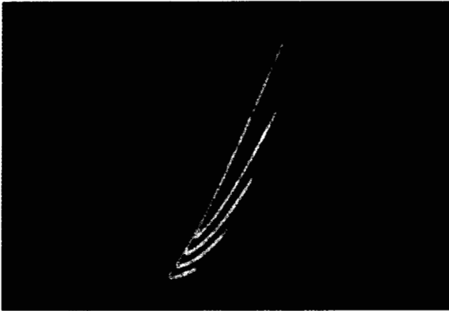
Fig. 29. Two-dimensional Poincaré section in the (voltage, current)-plane of the diode at E = 6.2 \text{ V} .
