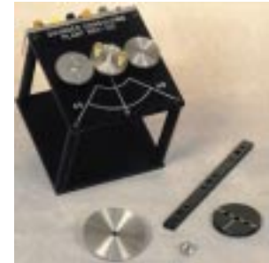
Figure 1.1 : SRV-02 shown in low gear ratio configuration and the gears required for high gear ratio configuration
