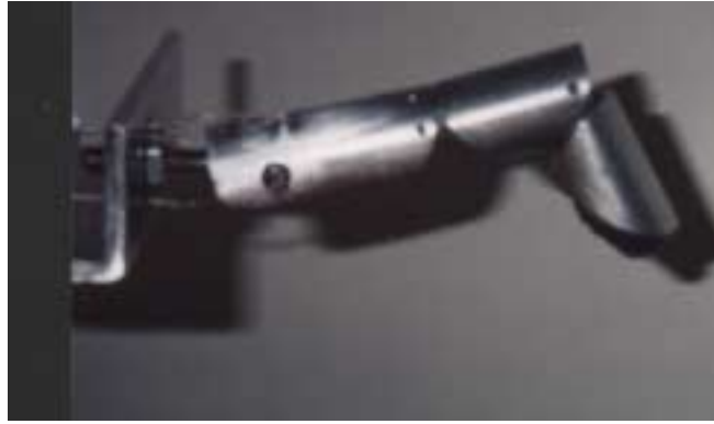
Figure 8. First Joint in Flexion
