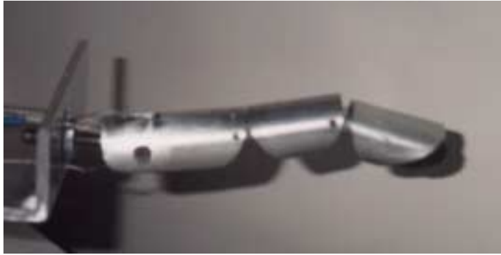
Figure 9. First Joint in Extension
