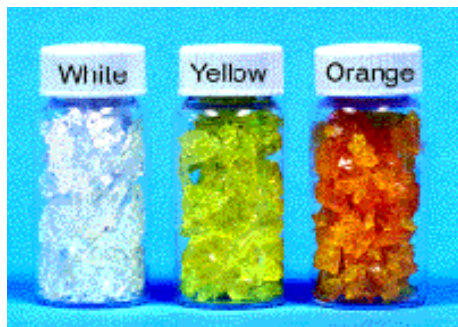
Figure 10.2. Nanoporous polymer samples in pure form (white), absorption of 4-nitrophenol (yellow), and absorption of 4-nitrothiophenol (orange) (reprinted from Li and Ma 1999; published 1999 American Chemical Society).
