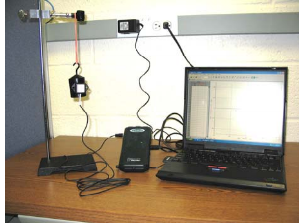
Figure 3—Damped Vibrations Experiment: Mass-spring (rubber band) system with accelerometer
