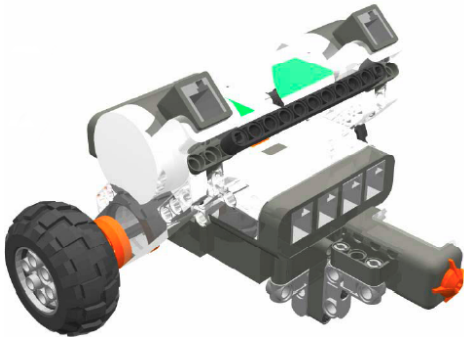
NXT Vehicle with Touch Sensor
