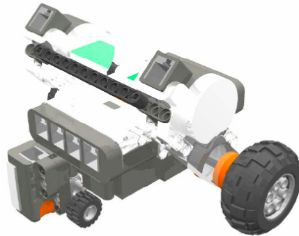
NXT Vehicle with Light Sensor
