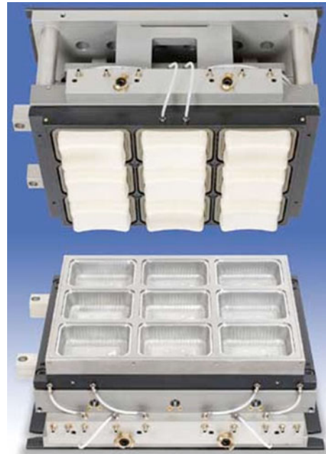
Fig. 15. Syntactic foam plugs used in thermoforming process. Images courtesy Jeff Barker, Tooling Technology LLC.
