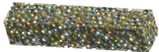
Fig. 4. Three-dimensional solid model representation of syntactic foams containing hollow particles. Image courtesy Dr. Dung D. Luong.
