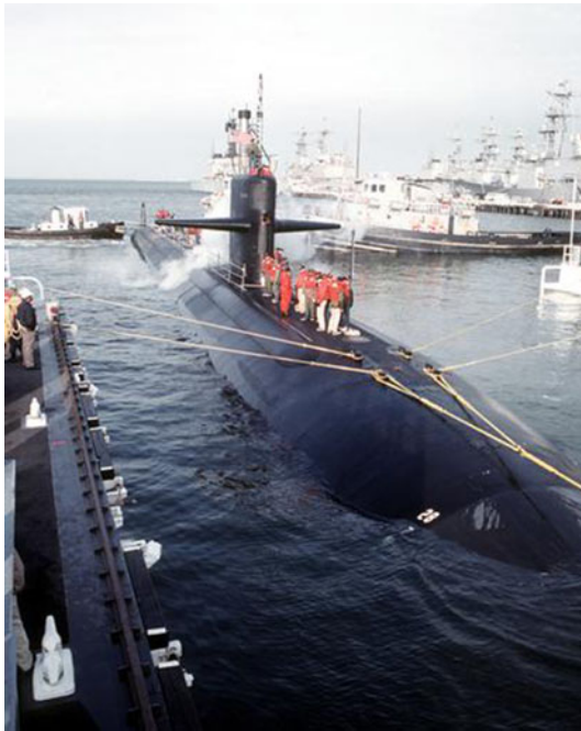
Fig. 10. USS Memphis nuclear submarine, which uses syntactic foams in its control surfaces and fairwater planes. 24
