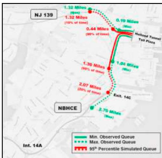
Fig. 3. 95 Percentile Maximum Simulated Queue Lengths in Base Case
