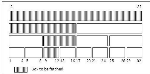
Figure 5: A 4-level stencil with b = 2 for a timeline of 32 days. The four shaded partitions need to be fetched for a query with range [9, 11].
