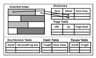
Figure 5.1: Major data structures in our index organization: standard (top) and additional structures in a fragment-based index (bottom).
