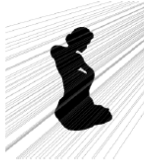
Figure 6: One object (top left) and its silhouette with 2D lines traced over it to find intersections along rays in the X , Y and Z ray-set of the MI, respectively. The number of lines has been reduced for illustration purposes: in typical cases they would cover most of the area of the image.
