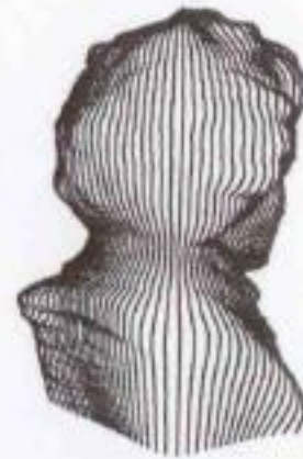
Figure 9.10: Left: Rear view of the recovered 3D profiles of the Beethoven statue shown on the left of Fig. 9.9, Right: Recovered triangular mesh around nose and mouth of the statue.
